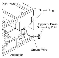
Figure 16 - Grounding Generator (Model RGH5500A Shown)
